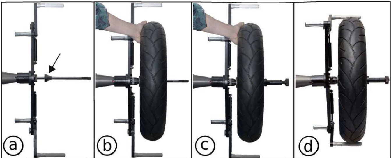
Fig. 5.13 Mounting motorcycle wheel on the holder.
