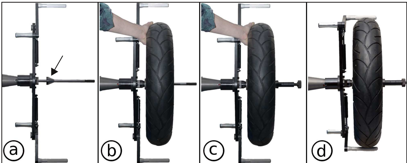
Fig. 5.13 Mounting motorcycle wheel on the holder.
