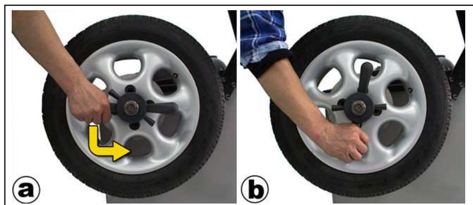
Fig. 5.8 Dismounting the wheel from the holder.
