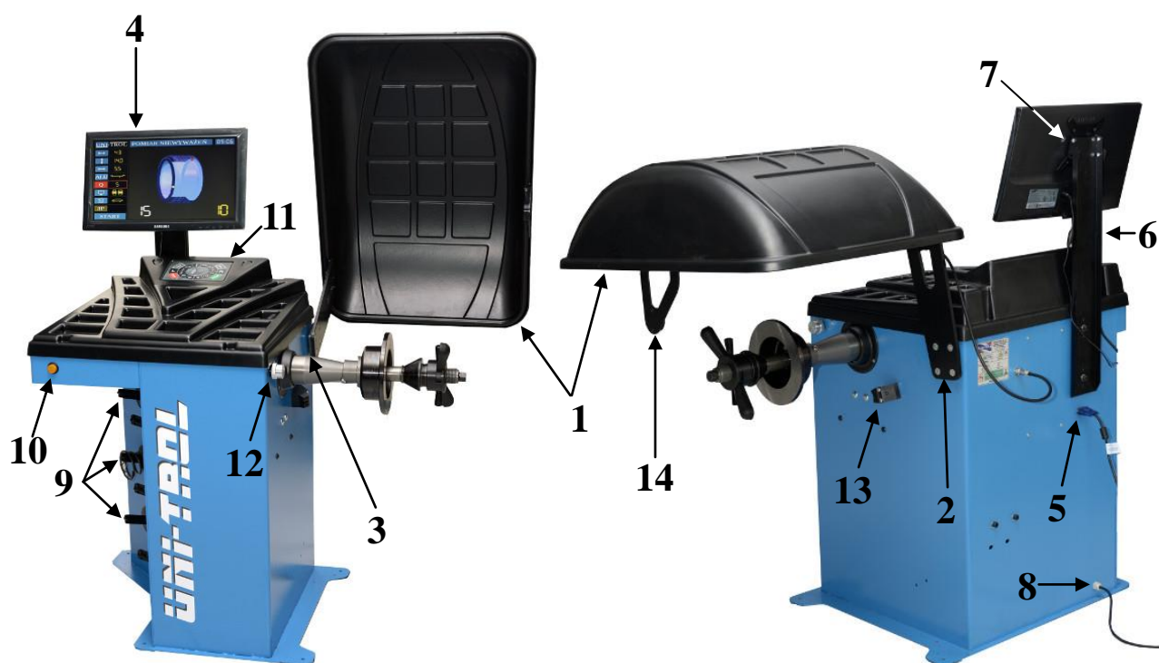
Fig. 2.1 Balancing machine – elements description
