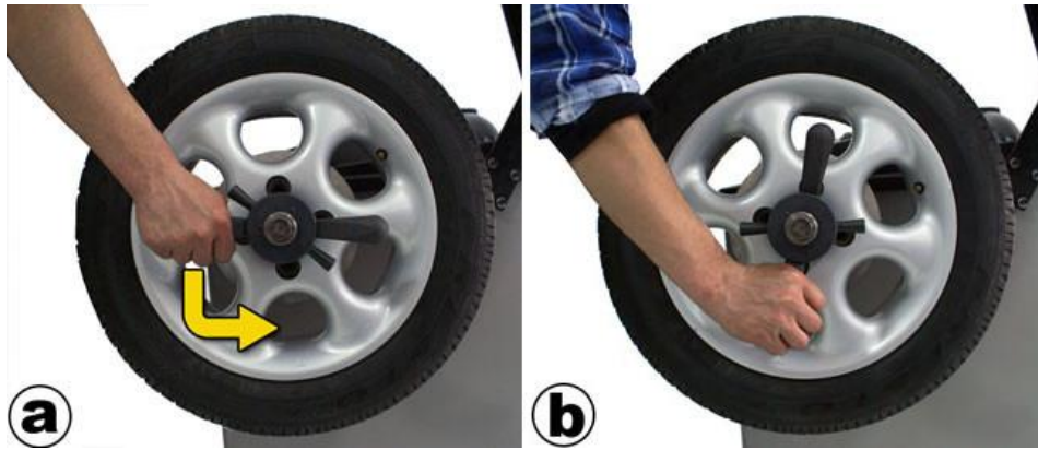
Fig. 5.8 Dismounting the wheel from the holder.
