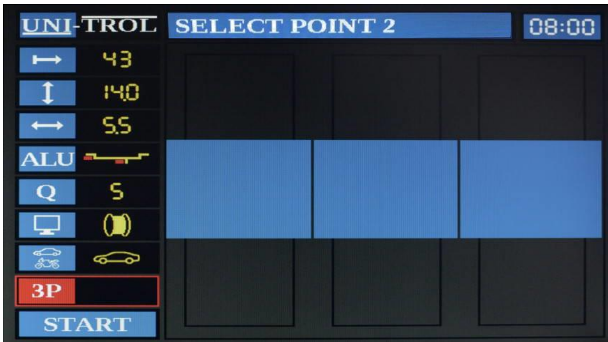
Fig. 6.6 – Screen of “hidden weight” function – selecting the second point.
