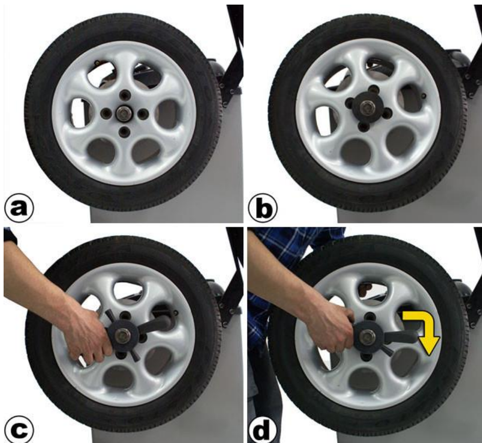
Fig. 5.7 Mounting a car wheel in the holder.
