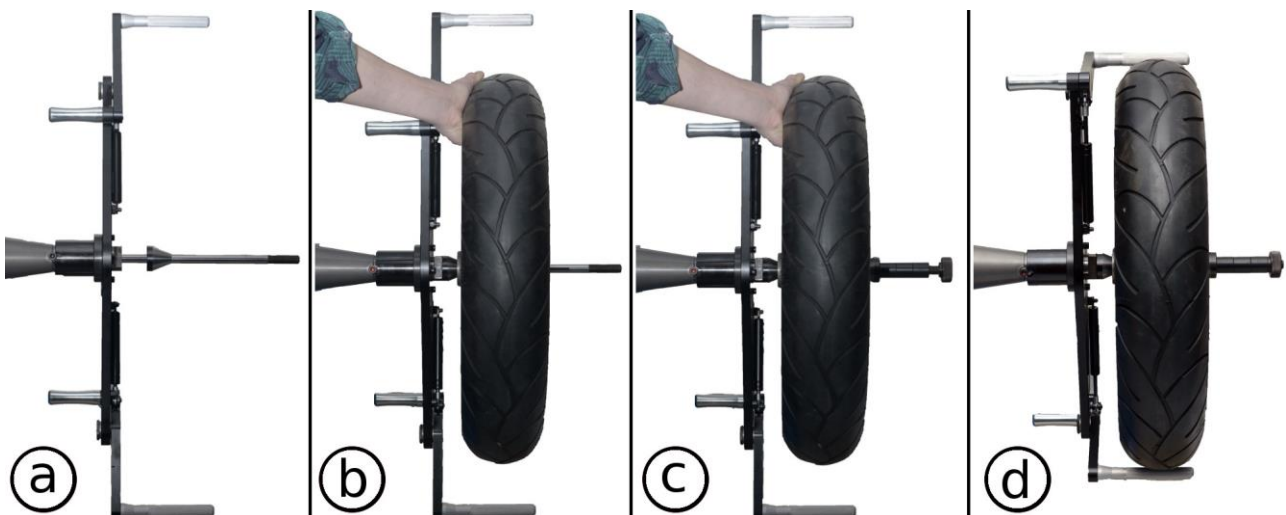
fig. 5.13 Mounting motorcycle wheel on the holder.
