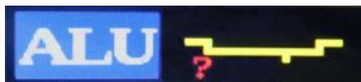
Fig. 7.6 The weight placement icon after first adjuster pull out for the automatic weight placement selection.
