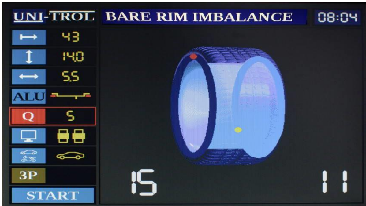
Fig. 6.11 – Optimisation screen – bare rim imbalance.
