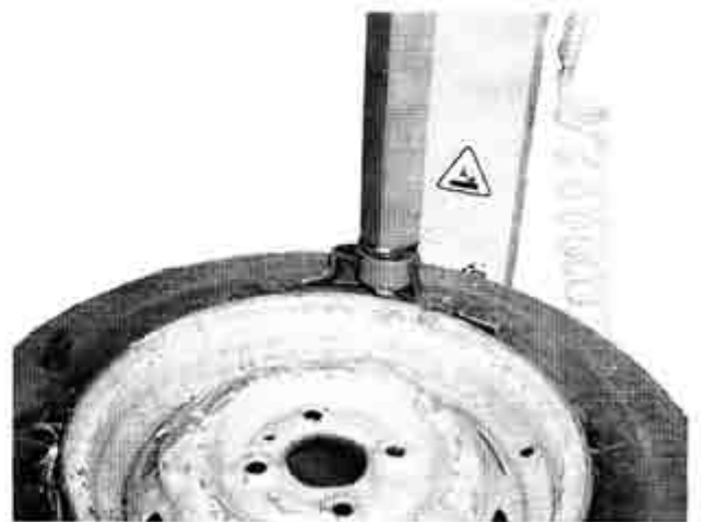
Fig. 9. Foot in operating position
